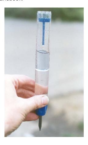
The picture illustrates the boundary between a considerable amount of water and the AVGAS below. Consider what to do with the sample; small amounts of petrol poured onto concrete will evaporate, but tarmac will be damaged. Do not consider returning samples to aircraft tanks unless they are completely free from contamination.
