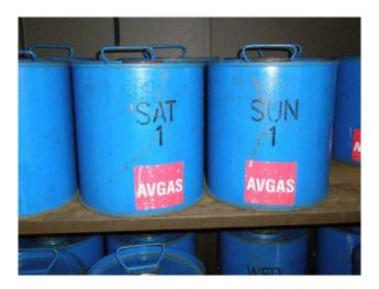
These should be marked with the date of sampling and kept cool and out of daylight, which can cause rapid deterioration of the fuel. After seven days, if they still appear in good condition, samples may be returned to the tank for later use, as may recycled hose contents.
